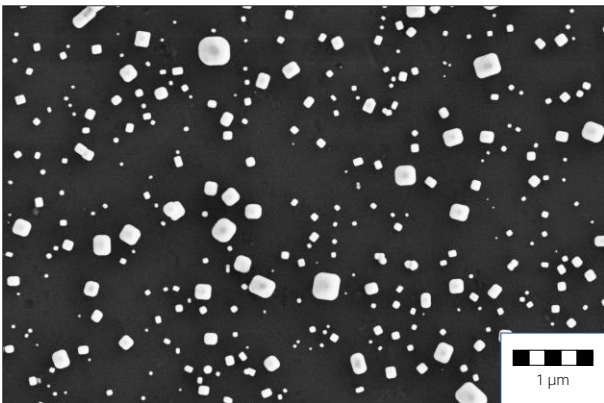
Scanning electron microscope image of electrostatically precipitated test aerosol particles generated by FCS 249 with commercial isotonic saline solution (0.9 wt-% NaCl).
