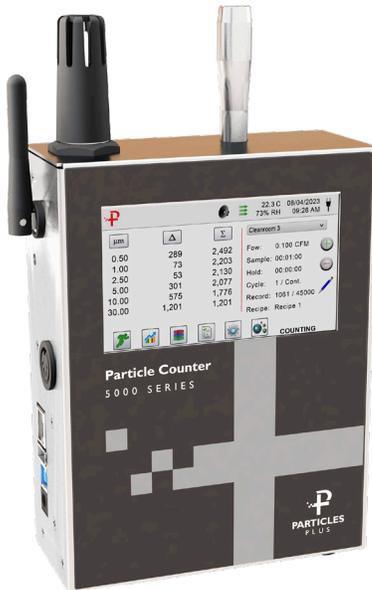
The Particles Plus® 5501P-30 Remote Particle Counter measures 0.5 to 75.0 µm and are the most feature advanced remote particle counters available. Integration is easy into a building automation and cleanroom management system via Ethernet, or (optional) Wireless 802.11 b/g, RS485 or RS232. Integrated web server displays instrument screen through any browser.
