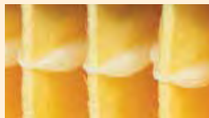
Adhesive beads bond the pleats into a rigid pack for even loading and complete media utilization.
